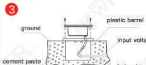
Put the power wire into plastic barrel and bury the plastic barrel with cement paste.
