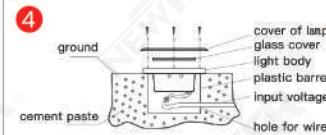
Input the glass cover to light body, and then use the screws and make the lamp cover with the lamp body tightly.
